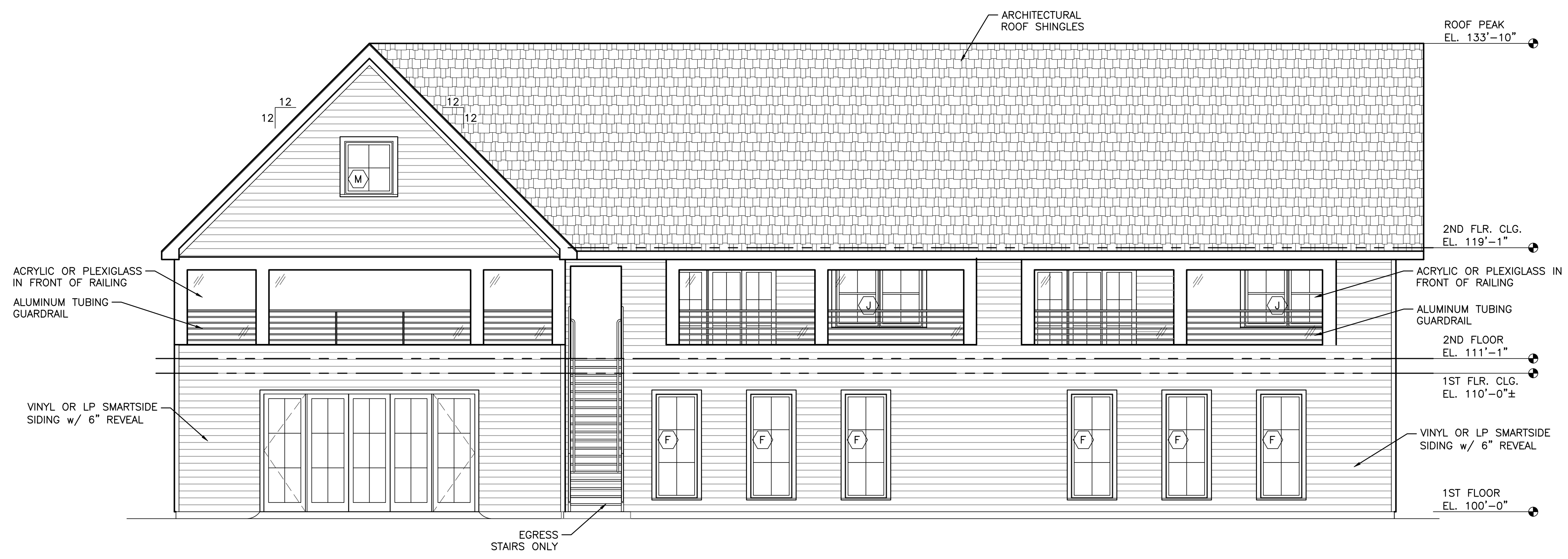
NORTH ELEVATION VIEW (5 A1) SCALE: 3/16" = 1'-0"
